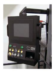
Computerized controls offer numerous benefits. Replacing relays and timers, manual buttons and switches with flat panel touch screen interfaces and innovative software allows thermoformers the ability to change every machine parameter within seconds. This eliminates the manual process of setting up different machine sequences, adjusting limit switches, opening and clos-
