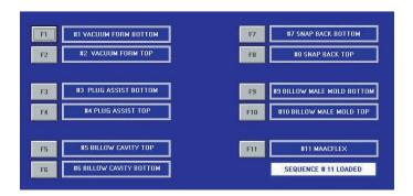
played on screen. The platen settings are then stored in the controller with each job for future recall. Although this has been available for quite some time, it is being taken further every year. Encoder driven platens no longer require homing or zeroing and the machine may be turned off without losing platen home position.
