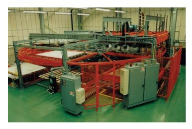
slide sheets onto the lift table instead of carrying or lifting sheets. Since the lift table also retrieves the formed part when the cycle is complete, the operator can also select what height he wishes to unload the part, once again making it easier on the operator.
